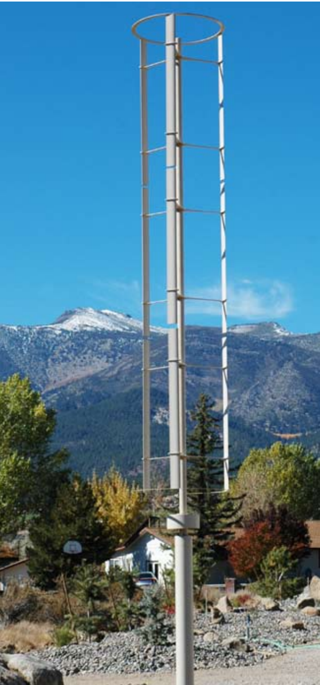
Designed by Reno resident Chris Gabrys, the Windspire can produce a third of a home's electricity needs.
